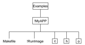
The resource files (such as !Run and Res) normally found in an application directory are not shown above. With directories arranged as above and default option settings, the work directories for both the Make and the CC/C++ tools are the same, namely Examples. !MyApp.
