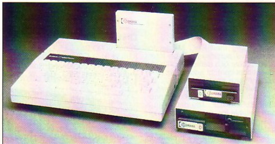
The Electron can run Disk User with 5" drives and a DFS chip. The Cumana system also offers a double density DFS option.
