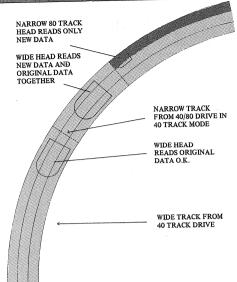
unit can read your programs that have been saved using a 40/80 track narrow head drive you should copy them onto a brand new disc that has never been written to with a wide head. Once a disc has had wide tracks laid down on it no amount of reformatting with a narrow head unit will clear the tracks completely.
