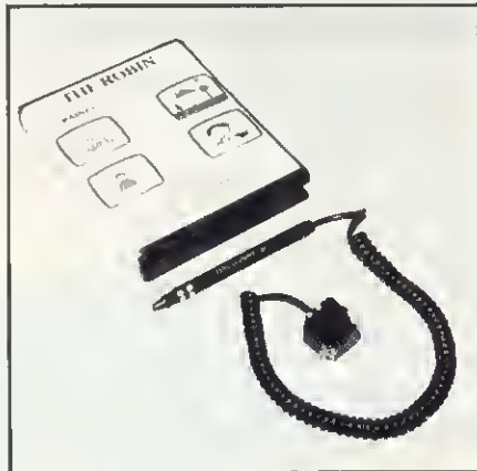
Figure 2. Lightpen, information cards and software cassette which make up the Robin Educational Light Pen package
