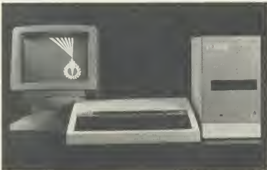
A Unix combination: monitor, Beeb and Unicorn box containing 68000 second processor, Z80 processor, 20Mb hard disc drive and 5¼in floppy drive
