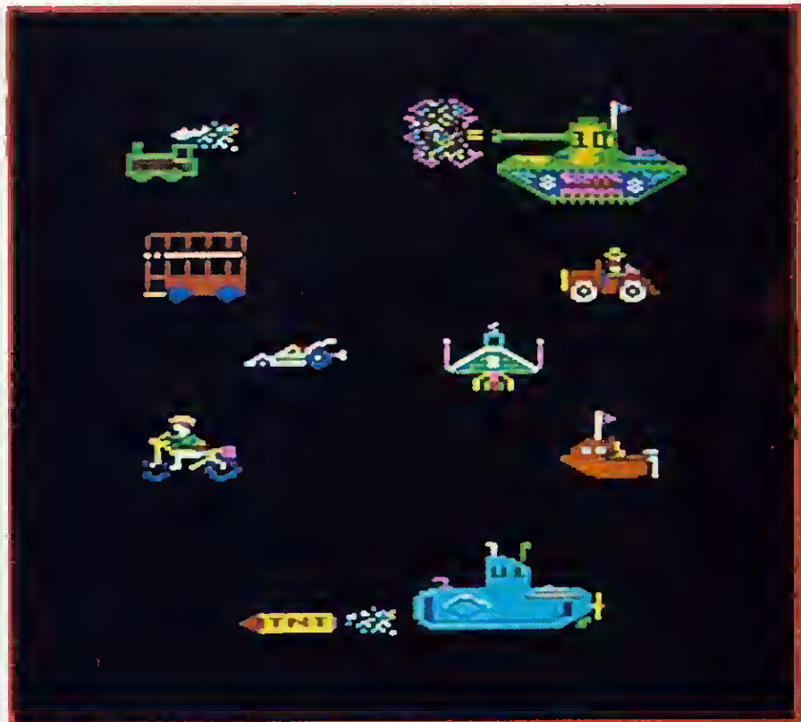
Some of the spritely characters from Harry Sinclair's portfolio. By combining four 'quartered' designs, such as the tank and submarine, a larger character can be created, and movement can be suggested with the use of flashing colours
