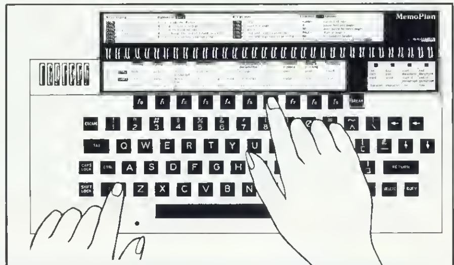
Diagram reproduced from the MemoPlan manual showing the function key strip booklet
