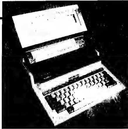
Sharp PC5000: this 128k, 16-bit machine has an 80-character by eight-line display and optional thermal printer running Superwriter software under MS-DOS. Options include 128k bubble memory packs, 64k expansion RAM modules, floppy disc drives, full range of MS-DOS software. Starting price £1195
