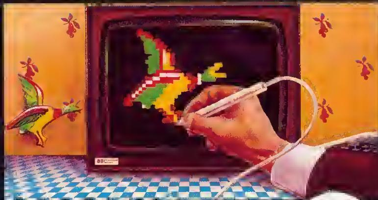
The lightpen is compact, reliable and comes in a rugged metal case providing physical and electronic protection. Its sensitivity can be adjusted to match any make of TV screen, giving the highest levels of accuracy.
