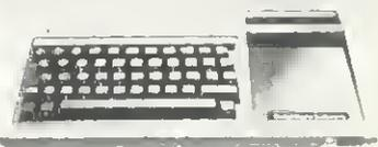
This microcomputer is based on TMS9900 16 bit microprocessor. It includes 16K RAM, 16 colour high resolution graphics (192 x 256). The screen display is 32 characters, 24 lines TI BASIC. Full size keyboard. For Software there are about 1000 programs to choose from. There are a lot of peripherals available, e.g. Disk Drive, Disk Interface, Speech Synthesizer, Extra RAM, Additional Language (PASCAL, LOGO, ASSEMBLER).
