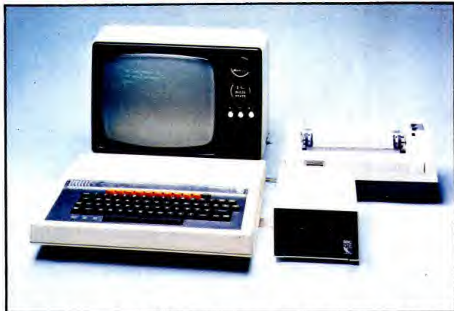
BBC micro with single disc drive and printer. The cover shows a BBC micro with a double disc drive.
