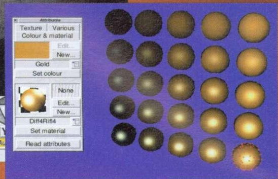
Figure 2: The attributes window allows properties to be assigned to objects, including the material type. This example, supplied with TopModel, shows the effect that changes in diffusion and reflection have on the appearance of a material
