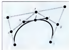
Drawing a bezier curve using a recursive sub-division method. All points e-j are mid points. Each sub-division generates one more point (j) that is guaranteed to be on the curve.
