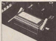
Figure 2. The NMC sideways socket installed. The board is attached to the underside of the keyboard cover with the sticky tape
