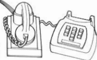
Modem or acoustic coupler links micro to phone (plugs into RS423 on the computer)
