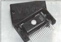
Figure 5. Inserting a ROM into the cartridge
