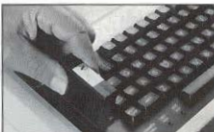
Figure 4. Inserting a cartridge into the Viglen socket
