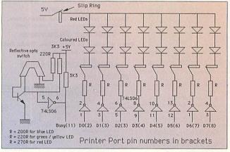
Figure 2: Preventing overloading the printer port
