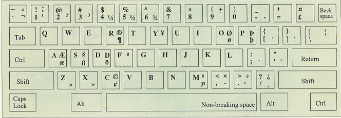
Figure 3: The standard RISC OS keyboard layout
