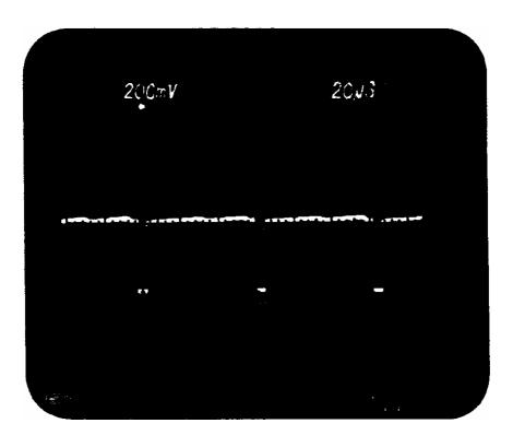
LINE SYNC with 10 to 1 scope probe
