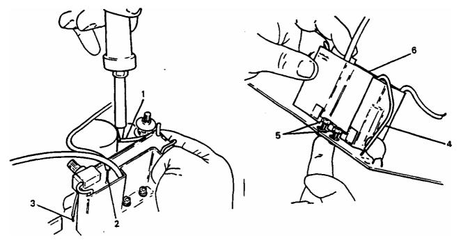
NOTE: Replace the insulation sleeve on connection (2)
