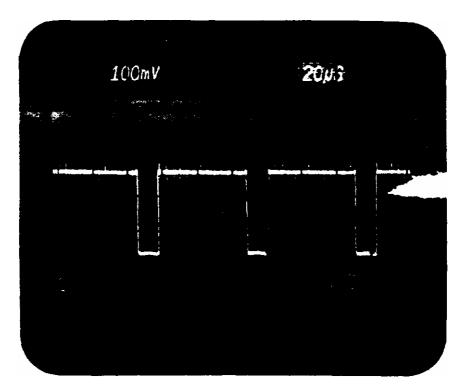
TR102 COLLECTOR with 10 to 1 scope probe
