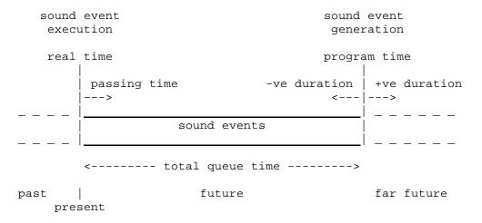
Durations move program time, and 'total queue time' is a measure of program time, relative to real time. The following words provide these functions: DURATION wait for a period of time number DURATION QTIME return queue time QTIME -> number Two further words have direct effects on the sound queue: READY get ready for players GO start players together Each player has its own independent program time. The system command line interpreter resets player 0's queue
