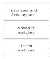
Both internal boundaries are movable. Modules are loaded from the bottom up, and when a module is loaded, the amount of memory available for the program is reduced accordingly.
