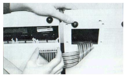
6 Plug it into the. socket marked 'tube' The grey retaining clips will click down when the plug is firmly in place
