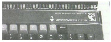
3 Position the cards so that the arrow on the page that you've put under the plastic strip points to the key marked f9
