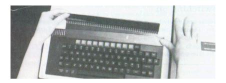
2 Hold the cards the right way up and push the back page under the strip, with the spiral binding at the top. The cards will now-be in position, with the back page under the plastic strip and the other pages lying on top of it
