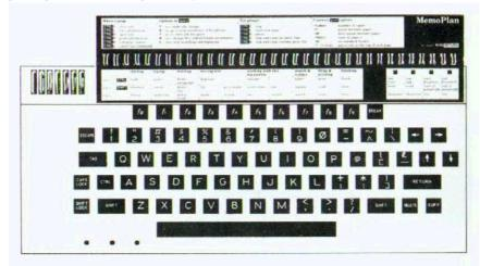
These key cards have been designed to stay permanently in position at the top of your keyboard, held in place by the clear plastic strip above the function keys. To fit the key cards in place:
