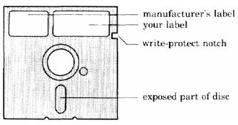
At the side of most discs is a notch, called the write-protect notch. This can be covered with a plastic adhesive patch which protects all the information on it from being wiped off by mistake. While this patch is on, you cannot save anything on the disc. You may wish to protect important discs you use, and you will find spare write-protect patches in your boxes of new discs.
