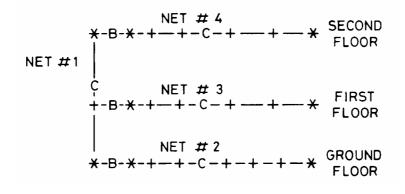
Where \* means terminator box + means socket box C means clock box
