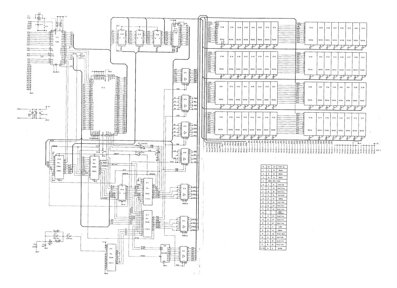
5.3 ARM co-processor circuit diagram
